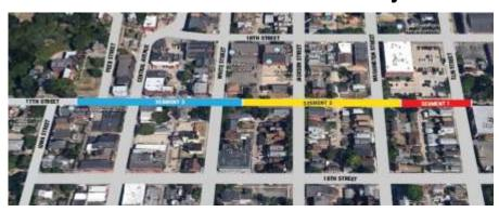
You may have noticed the work being done on 17th Street right by the church. This is part of the Bee Branch extension project. The purpose of this project is to increase the capacity of the storm sewer from the Lower Bee Branch Creek up 17th Street to West Locust Street. A larger storm sewer and additional high-capacity storm drains will help alleviate the flash flooding frequently experienced on these streets. The estimated completion date of the entire project is 2021.
